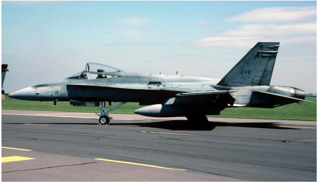
This is a photograph of Cf-18 188741 which was involved in attacking an Iraqi Patrol boat on January 30, 1991. The CF-18 was a modern fourth generation air superiority fighter. It had nine external hard points carrying air to air missiles, bombs and external fuel tanks. It also had a 1x20mm M61A1-Vulcan internal rotary cannon. Maximum speed was 1,127 mph (1,814 km/h), combat range was 330 miles (540kms) and it had a service ceiling of 50,000' (15 000m).
