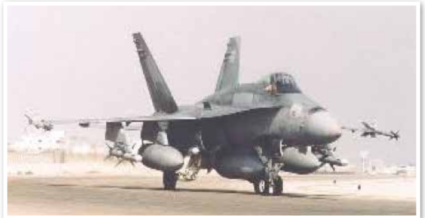
The CF -18 Hornet is a multi- role fighter. With two General Electric F404-GE-400 low bypass turbofans it can produce 16000 lbs. of thrust and is capable of Mach 1.8. Notice the AIM-9M Sidewinder and AIM-7M Sparrow missiles.
